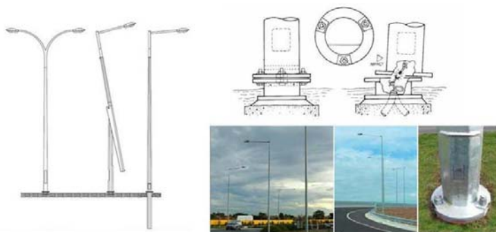
Figura 23: Stâlpi de tip “rupere de la bază” (Source: Department of Infrastructure, Energy and Resources: Road Hazard Management Guide, Tasmania, 2014)
